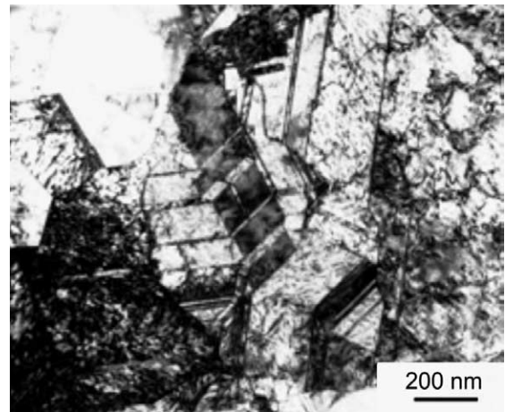
Fig. 5. TEM image of an indented Cu sample with high twin density.
