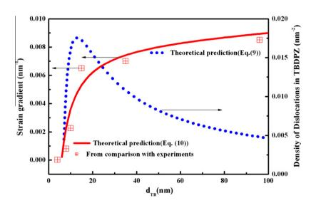
Fig. 9. The local strain gradient in the TBDPZ as a function of twin spacing obtained from the comparison between experiments and model predictions. Also shown in the plots are the corresponding fitting curves based on Eq. (10), and the curve of the dislocation density in the TBDPZ varied with twin spacing calculated from Eq. (9).
