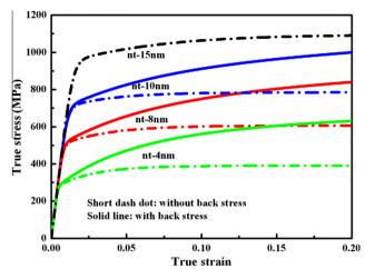
Fig. 8. Stress-strain curves for cases in which the effect of back stress on strain hardening is switched on (solid lines) or off (dashed lines) for twin spacings of 15, 10, 8 and 4 nm.
