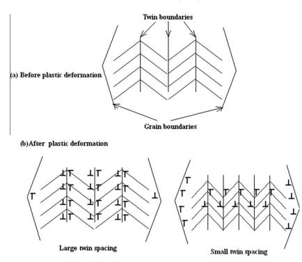
Fig. 4. Schematic drawings of dislocations piled up along the TBs and those that stop at the GBs. For a large twin spacing, a large number of dislocations are stored along the TBs and few dislocations stop at the GBs. In the case of a small twin spacing, the dislocations along the TBs vanish and the number of those that stop at the GBs increases, providing for the kinematic strain hardening in the nanotwinned metal.
