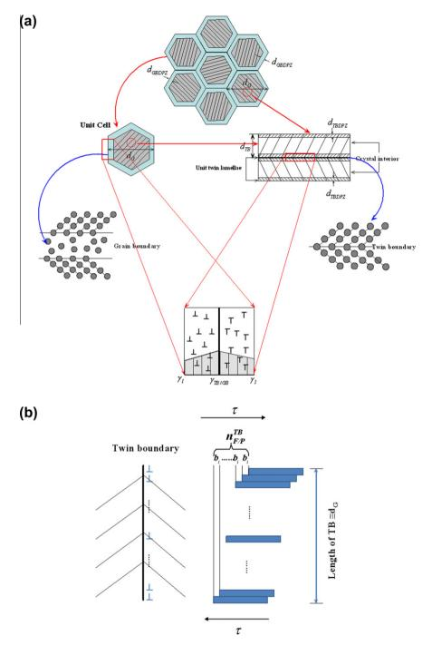
Fig. 2. (a) Schematic drawings of the proposed model for nanotwinned polycrystalline metal in which the TBDPZ and GBDPZ are introduced. (b) A schematic illustration of shear strain originated from dislocation accumulations in the TBDPZ in which  $\mathbf{b}_i(i = \mathbf{F}, \mathbf{P})$  is the magnitude of the Burgers vector for full dislocation and/or partial dislocation.
