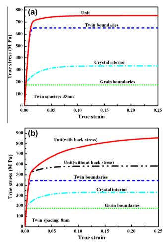
Fig. 7. The separate strengthening contributions associated with dislocations in the TBDPZ ( $\sigma_{flow} = M \alpha \mu b \sqrt{\rho_{TB}}$ ), the GBDPZ ( $\sigma_{flow} = M \alpha \mu b \sqrt{\rho_{GB}}$ ) and the crystal interior ( $\sigma_{flow} = M \alpha \mu b \sqrt{\rho_1}$ ), and those associated with back stress for two selected cases in which twin spacing is taken as 35 nm and 8 nm.
