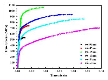
Fig. 1. Tensile stress-strain curves for as-deposited nanotwinned copper samples with mean twin thickness varying from 96 to 4 nm [10].
