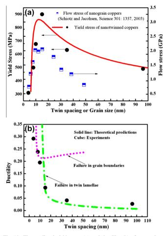
Fig. 10. The predicted yield stress (a) and ductility (b) of nanotwinned copper as functions of twin spacing in comparison with the corresponding experimental results. The lines are the predictions and the circles are the experimental data.
