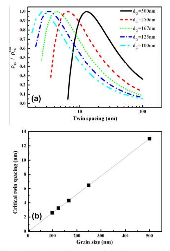
Fig. 11. (a) The density of dislocations in the TBDPZ as a function of twin spacing with different grain sizes; (b) the critical twin spacing as a function of grain size in the nanotwinned polycrystalline copper.
