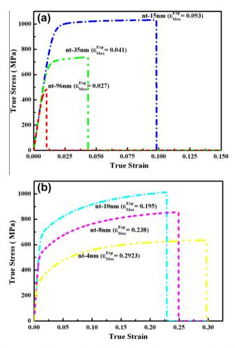
Fig. 6. Predictions for the ductility of nanotwinned copper with twin spacing ranging from 96 to 4 nm. The failure mechanism in the twin lamellae dominates the elongation process for large twin spacings (a) and the failure mechanism in the GBs becomes dominant over the failure mechanism in the twin lamellae for twin spacings less than 15 nm (b).
