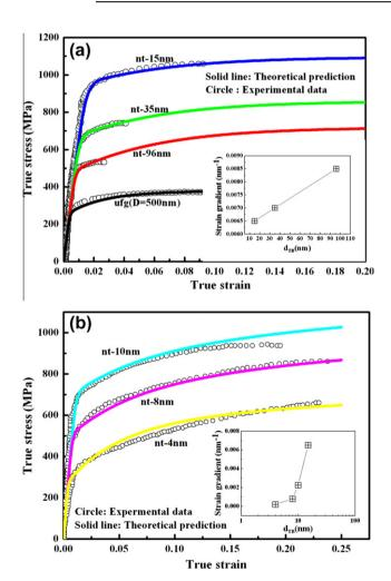
Fig. 5. (a) Simulated vs. experimental [10] tensile stress–strain responses of nanotwinned ultrafine-grained copper with twin spacings of 96, 35 and 15 nm and of ultrafine-grained copper free of twins. (b) Simulated vs. experimental [10] tensile stress–strain responses of nanotwinned ultrafine-grained copper with twin spacings of 10, 8 and 4 nm.
