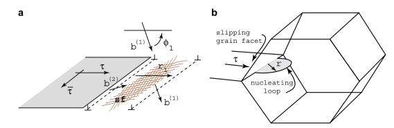
Fig. 11. (a) A model for partial dislocation emission from a grain boundary that acts in a crack-like manner. The crack is loaded via an in-plane Mode II applied stress,  $\tau$ , and an anti-plane Mode III shear stress,  $\bar{\tau}$ . (b) Nucleation of a partial dislocation loop at the front of a freely slipping grain boundary facet. (Figure taken from Ref. [127].)
