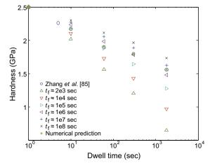
Fig. 13. Simulated hardness vs. time [93], compared with the measurements of Zhang et al. [85]. The simulations were performed using a wide range for  $t_{\rm f}$ , i.e.  $2 \times 10^3$  s  $\leq t_{\rm f} \leq 10^8$  s. (Figure taken from Ref. [93].)
