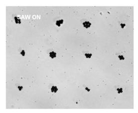
Movie S3. Three-dimensional trapping and manipulation. This movie corresponds to Fig. 5C. Here, 10.1-µm-diameter polystyrene particles were captured and suspended into a single layer of 3D trapping node arrays (in the focus plane), transported along the *y* axis, and deposited onto a substrate along the *z* direction (as the particles move out of focus) while maintaining the array formation. The movie is in real time. (Scale bar: 100 µm.)
