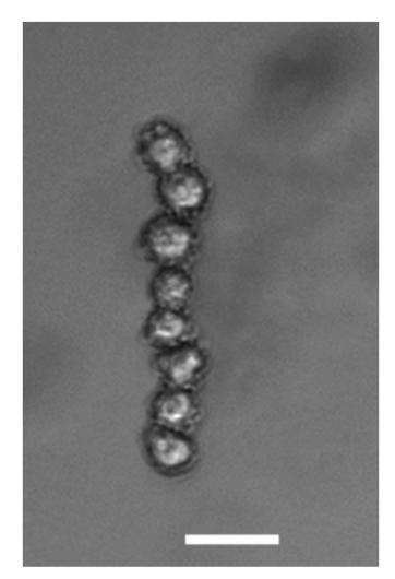
Movie S4. Acoustic-based cell rotation. The entire HEK293 cell chain was trapped and rotated under the applied acoustic field. The movie is in real time. (Scale bar: 20 µm.)
