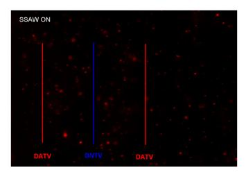
**Movie S1.** Acoustic streaming (1D SSAW). This movie corresponds to Fig. 3C. Here, 1- $\mu$ m-diameter red fluorescent polystyrene particles are used to trace the flow of the acoustic vortices close (40  $\mu$ m above) to the substrate surface. The movie is in real time. (Scale bar: 50  $\mu$ m.)
